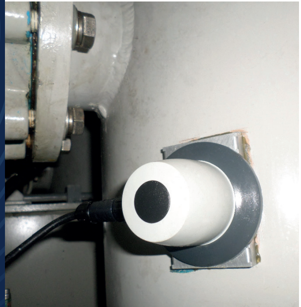
Single transducer fitted with bracket on a sea chest pipe.
